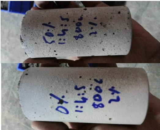
Figure 3. Specimens after exposure to 800 0 C with 2%ZrO 2
