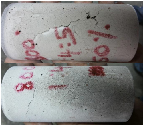
Figure 2. Specimens after exposure to 800 0 C with 0%ZrO 2
